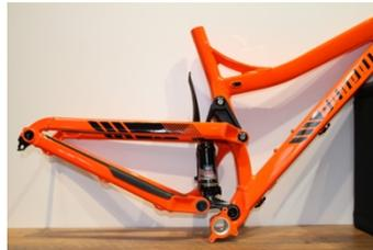
Clean the running surface of the shock after every ride, especially in extremely dusty or muddy conditions. Lubricate the seal at the piston rod according to the manufacturer's instructions.
