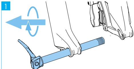
Remove the thru axle from the fork.
