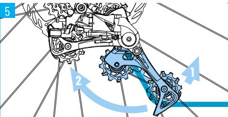
Deactivate the Cage Lock function. Pull the cage of the derailleur slightly forward and carefully return the derailleur to its original position.
