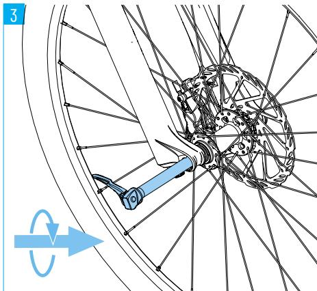
1. Put the front wheel into the dropouts of the fork. The brake rotor must be placed between the brake pads.
