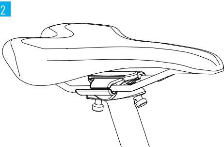
1. Attach the upper clamp to the saddle frame.
