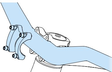
1. Attach the handlebar to the stem.
