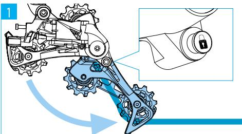
Activate the Cage Lock function. Pull the cage of the rear derailleur forward and press the Cage Lock button with the symbol
