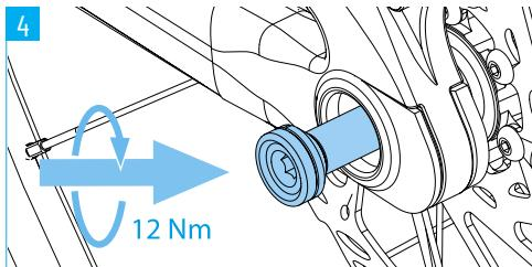
Screw the thru axle into the dropout using a 6 mm hex key and tighten the thru axle to a torque of 12 Nm.
