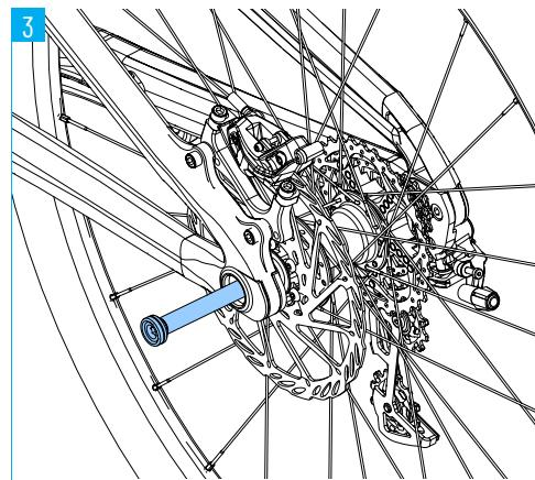
1. Insert the rear wheel into the dropout of the frame.
