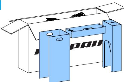
Remove the fixation of the handlebar, the fixation of the rear triangle and the fixation of the fork.
