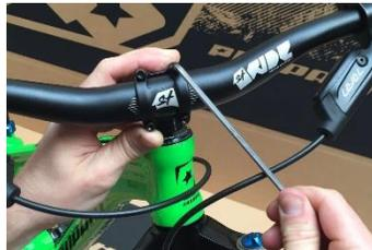
3. To mount the handlebar to the stem you first need to remove the front cap from the stem. When attaching the handlebar to the stem, make sure to mount it in the correct position and pay special attention that all the cables are routed smoothly around the frame. Finally, put the cap around the handlebar and tighten the bolts with the correct tightening torque (6Nm - use a torque wrench). The scale on the handlebar helps you to adjust it precisely.
